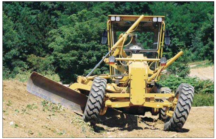
**Blade positioning.** The blade linkage design provides extensive moldboard positioning. This extended range is most beneficial in mid-range bank sloping and in ditch cutting and cleaning.
