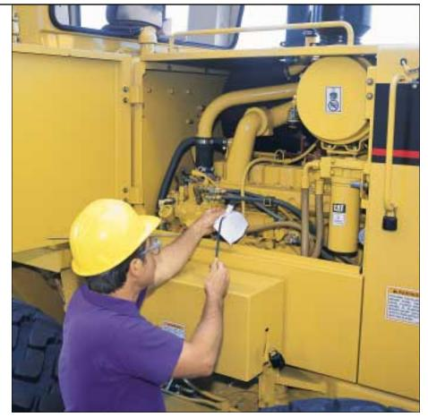
**XT hose.** Caterpillar designs and manufactures its own heavy-duty XT hose and installs it in all highpressure circuits. Its resistance to abrasion, coupled with its exceptional strength and flexibility, help minimize maintenance and extend life.
