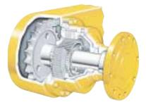
**Power shift transmission.** Caterpillar designs and builds transmissions specifically for Cat motor graders. The transmission provides on-the-go, full-power shifting as well as inching capability.
