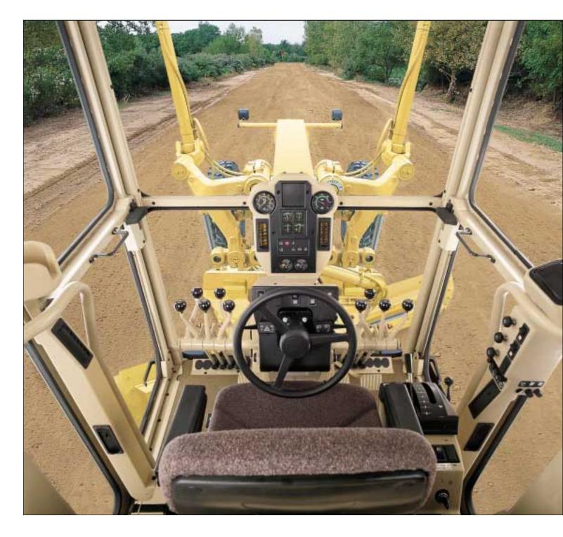
**Exceptional visibility** helps improve operator confidence and productivity. The drawbar has been modified to improve the view through the circle, allowing the operator to see the material as it rolls along the moldboard without leaning. Large side windows allow a clear view of the moldboard heel and tandem tires. A wide rear window and tapered engine hood provide a good view to the rear of the machine.
